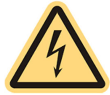
Figure 1: Marking of voltage class B components and circuits
